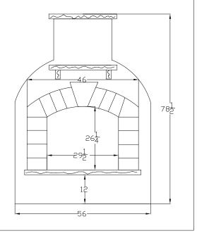
Dimensions above are in inches. Reference dimensions only. We recommend measuring individual units at installation. Refer to installation manual for detailed specifications on installing this product.
